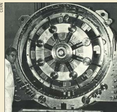
The rotary condenser of the r.f. acceleration system for the SC improvement programme in its vacuum housing, with the end shield removed. The eight symmetrically placed electrodes couple the condenser to the oscillator valve via the coaxial feed (centre).
