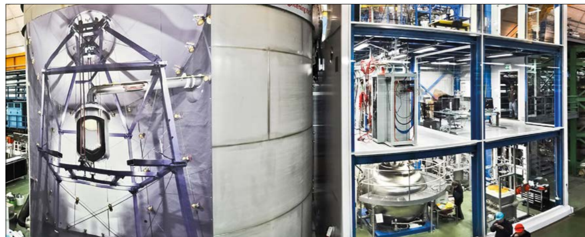
Fig. 3. The XENONIT detector. Left: The water Cherenkov veto with cladding, showing the cryostat and its support structure inside. Right: the service building with cryogenics, purification, storage and recovery systems, as well data acquisition and slow control.
